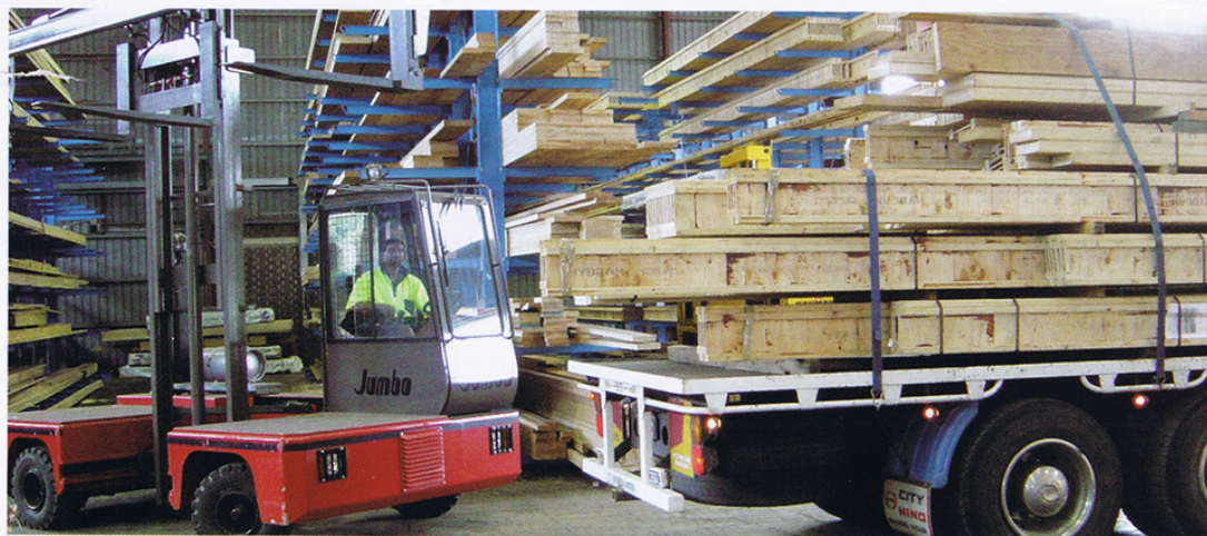
Handling a complete range of stock, Swan Le Messurier has installed a new sophisticated rack storage system and purchased side loading equipment.
